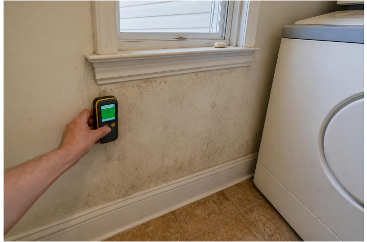
Interior 8.1b - Moisture meter location at the stained laundry wall below the rear window.
